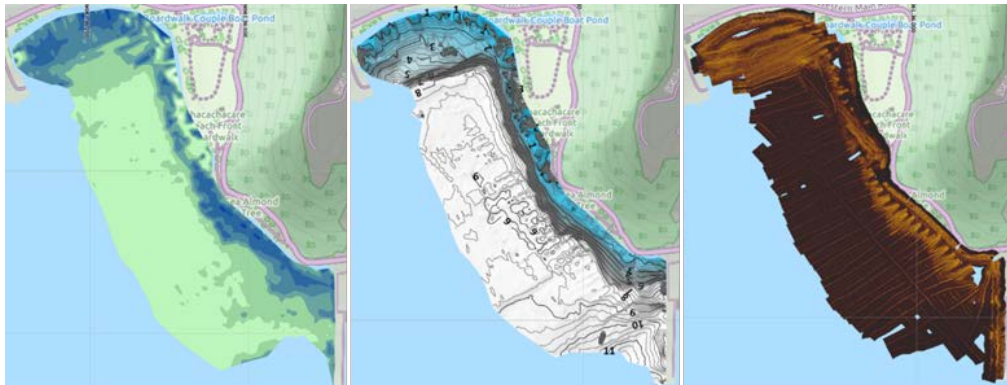
Fig. 1. From left to right: roughness map (E1), bathymetry map (0-11 m) and SSS mosaic for Williams Bay, Trinidad.
